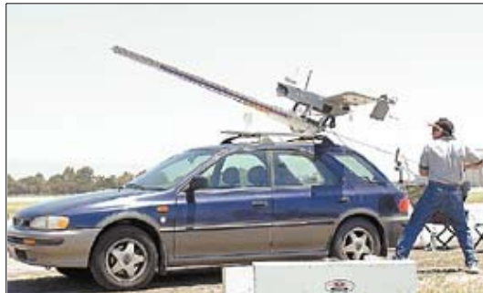
NASA Ames Research Center / Associated Press Steve Morris prepared to launch the MLB Bat, an unmanned aerial vehicle, from atop a car at Moffett Field near Mountain View last month. UAVs have been tested for firefighting use.
