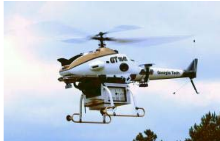
GT Max, the first rotary wing UAV, is able to learn as it flies, maneuver aggressively and automatically plan a route through obstacles thanks to its Open Control Platform system. (Photo courtesy of Georgia Institute Of Technology)
